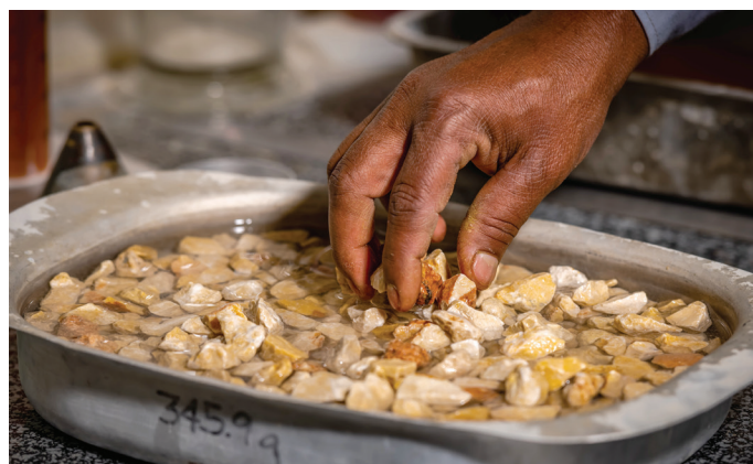
Al Kifah also offers mixes utilising recycled metal slag aggregates.
